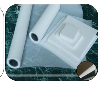
**PURE PTFE SHEET** has excellent resistance to the majority of chemicals and solvents and is capable of operating at high and low temperatures. It also has a very low coefficient of friction and is commonly used in food contact applications. It provides good thermal stability and has good electrical properties, but is not suitable for wear application and is difficult to bond.
